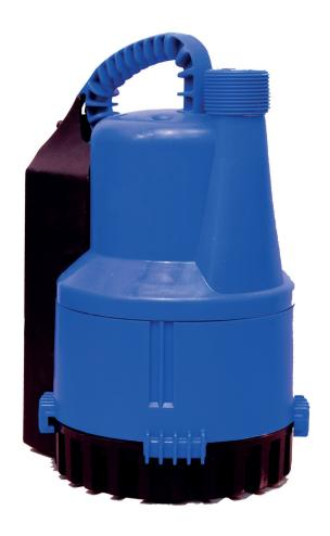
The R202 has been designed for fixed or transportable installation, and for internal or external applications such as emptying containers and drainage pits, draining of swimming pools, kitchen waste or flooded cellars. Plug-in, submersible pump, for the removal of waste water containing solids up to 10mm.
