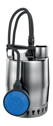
The KP250 is a 230V stainless steel automatic submersible pump with a 10 mm clear opening. Its semi-open impeller is suitable for ground, surface, storm and grey water applications.
